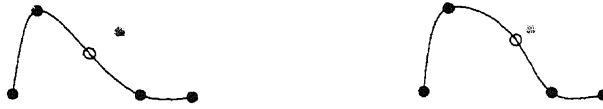
Fig. 3. Left: original curve and a point attractor. Right: resulting constrained variational curve.
