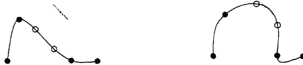
Fig. 4. Left: original curve and a curve attractor. Right: resulting constrained variational curve.
