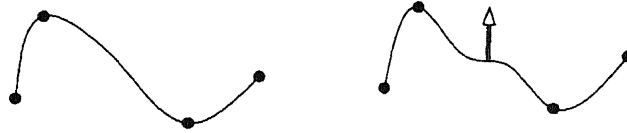
Fig. 1. Left: variational curve with point interpolation constraints. Right: variational curve with normal constraint.
